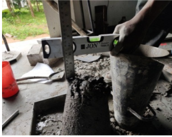
Fig. 7. Slump Tests
