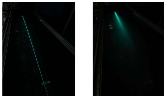
Fig.1. Laser in water containing different amount of scattering agent.
