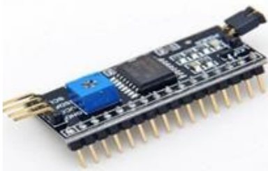
Figure 8 i2c LCD Module (PCF8574)
