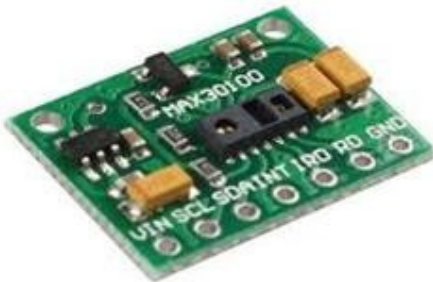
Figure 3 MAX30100 Sensor
