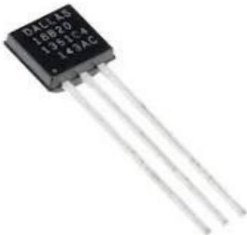
Figure 4 DS18B20 Temperature Sensor
