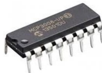
Figure 6 ADC(MCP3008)
