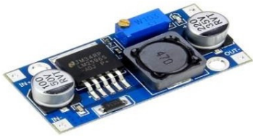
Figure 11 LM2596 Buck Converter
