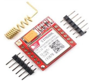
Figure 9 GSM Module (SIM800L)
