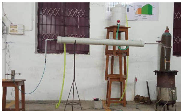
Figure.1 Pyrolysis Batch Reactor
