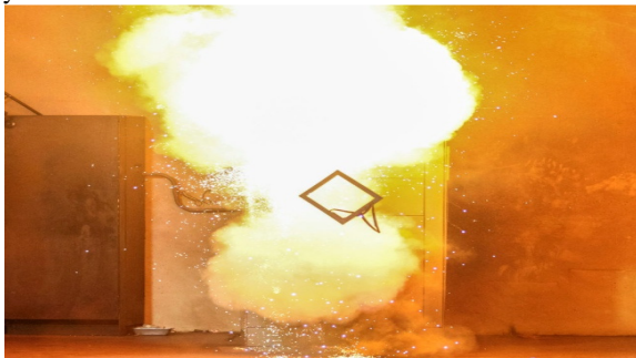
Fig. 3 Fire Explosion in electric supply board
