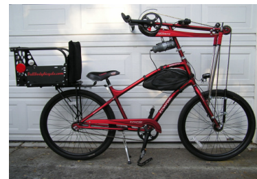
Fig.III.F. Full body bike (can be operated by both hands and legs at the same time and separately) (Source: https://energonplus.ru/aGFuZCBwZWZRhbCAgYmlrZQ/ )
