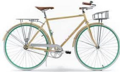
Fig.III.A. A classical bicycle with rear wheel drive – single ratio (Source: https://www.fixedgearfrenzy.com/products/state-bicycle-co-city-shoreline-deluxe )
