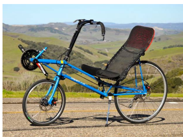
Fig.III.D. Short wheel base recumbent bicycle with crank in front of the front wheel (Source: http://www.lightningbikes.com/p38/ )
