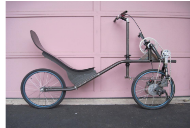
Fig. III.E. A recumbent bike - front wheel drive with U joint (Source: Benjamin Knaus, Philip Basmadjian, Nick Supat, ASME Human Powered Vehicle, A thesis submitted to the faculty of the Mechanical Engineering, California Polytechnic State University, (2010))
