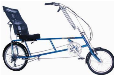
Fig.III.C. A recumbent bicycle with midway pedal (Source: Aleah Pavlicek, Brandon Walker and Xingyu Chen, Terence Staples, Quamrul Mazumder, Design and Improvement of a Human Powered Vehicle (HPV))
