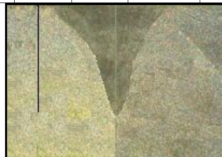
Fig.8 MI Sample 3 Butt Joint : 100W
