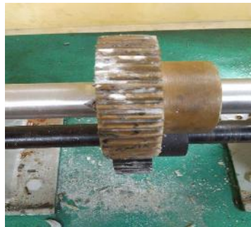
FIGURE 5 DEFORMATION OF GEARS FOR 15%: BEFORE WEAR AND AFTER WEAR
