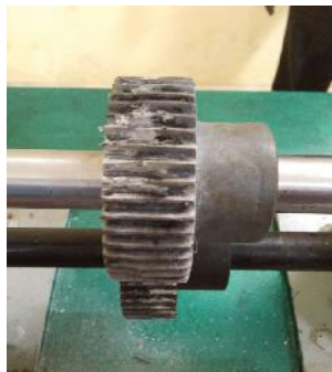
FIGURE 6 DEFORMATION OF GEARS FOR 20%: BEFORE WEAR AND AFTER WEAR
