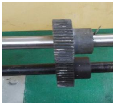
FIGURE 5 DEFORMATION OF GEARS FOR 15%: BEFORE WEAR AND AFTER WEAR
