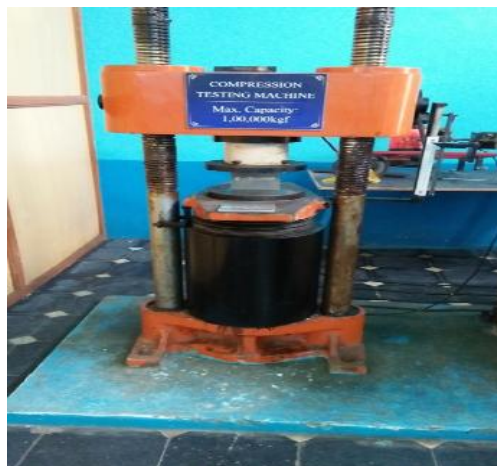
Fig 10 Compression testing machine
