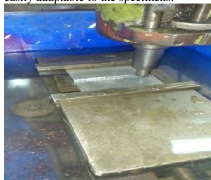
Fig 5 position of FSW tool while machining
