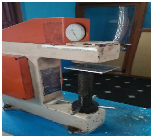
Fig 9 Rockwell hardness Testing machine
