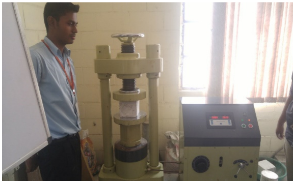
Fig 3.2 Compressive Strength Test (Cubes 150x150x150mm)
