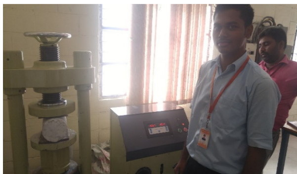
Fig 3.4 Split Tensile Strength Test (Cylinder 150mm dia and 300mm height)
