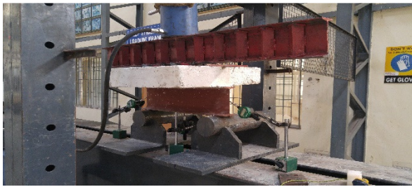
Fig 5.1 Shear connector welded composite beam
