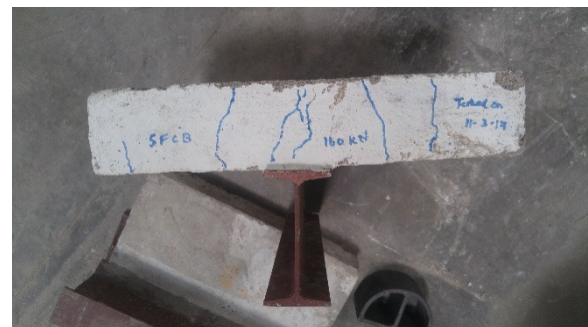
Fig 5.6 Crack pattern of Ferro cement self-compacted concrete composite beam
