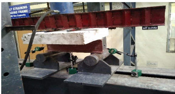
Fig 5.3 Shear connector welded Ferro cement composite beam
