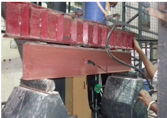
Fig 5 back to back channel section
