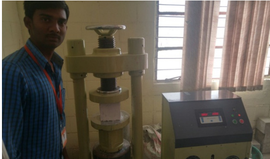
Fig 1 Compressive Strength Test
