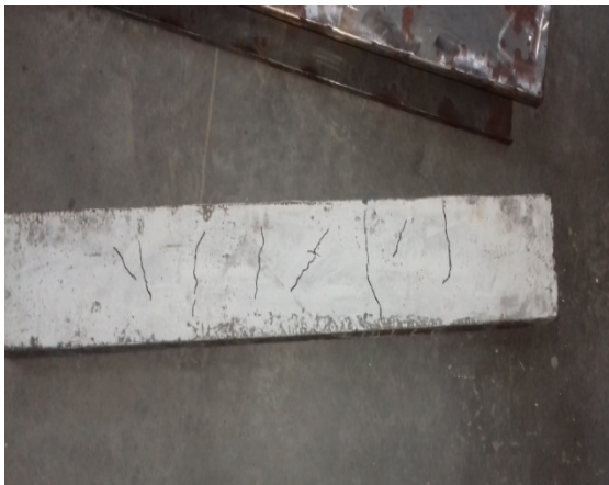
Fig 10 crack pattern in encased beam
