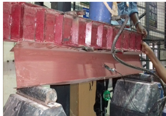
Fig 7 failure of back to back channel section
