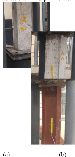
Fig6. Failure Pattern (a) Proposed Composite column, (b) Conventional RC Column, (c) Conventional Steel Column
