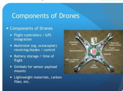
Figure 13: components of a common UAV.
