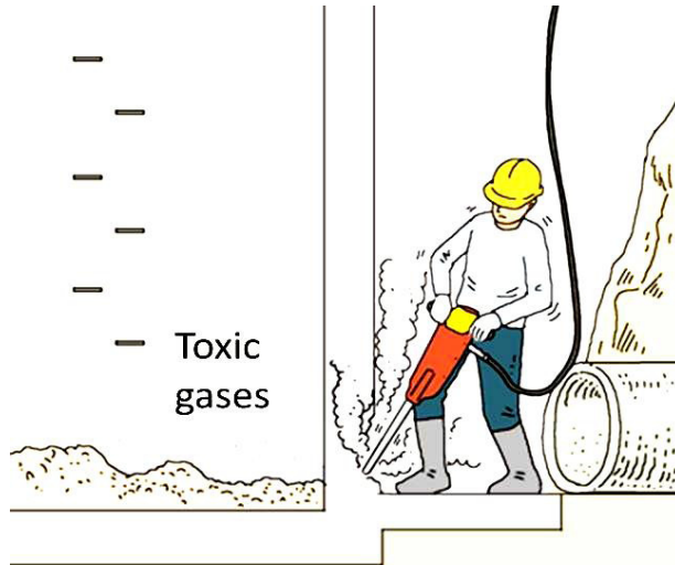
Figure 2: Disregard the risk of sudden ingress of toxic gases as a result of the engineering work
