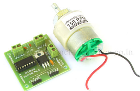
Figure7: Motor Driver Circuit
