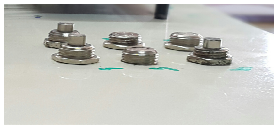
Fig 5- Actuated Braille Pattern for the letter 'm'.
