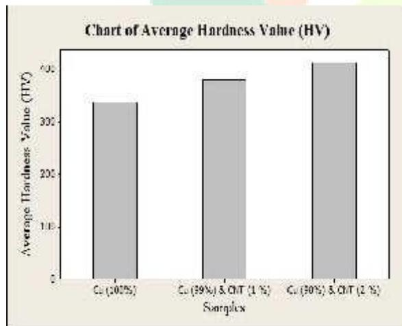
compacting green composite pieces are sintered in presence of Argon gas at 900°C. Micro hardness of the composite determined by Vickers hardness indenter using 0.3kgf load and 5sec dwell time. Corrosion test carried by salt spray method.
