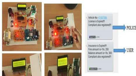
Our project contains RFID reader and RFID tags (vehicle insurance, driving license) whenever the tag is shown in front of the reader it will read the data from the tag, if it is valid it will display on LCD as valid otherwise the buzzer will buzz. Additionally, we are having alcohol sensor to identify whether the person is in drunk and drive or not. This process helps the user and police department to verify the documents of the vehicles whether the particular data is correct or not.
