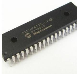
The specification of microcontroller is 16F877A. It belongs to high performance RISC family. It means that 16 refers to serial number, F means Flashable, 8 refers to 8 bit, 77 is a product
