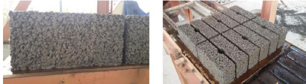
Casting of No Fines Bricks
