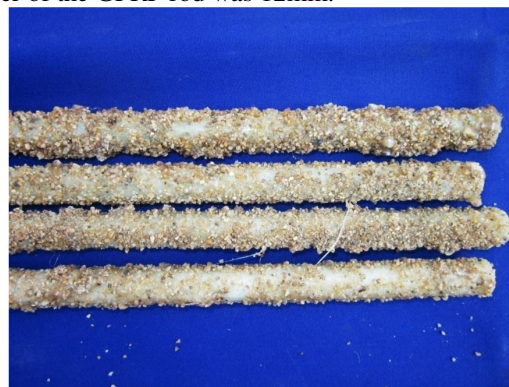
Fig 2 Sand sprinkled GFRP rebars
