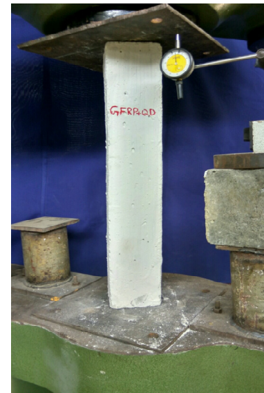
Fig 4 Test Setup of column
