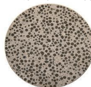
Self healing bacterial concrete
