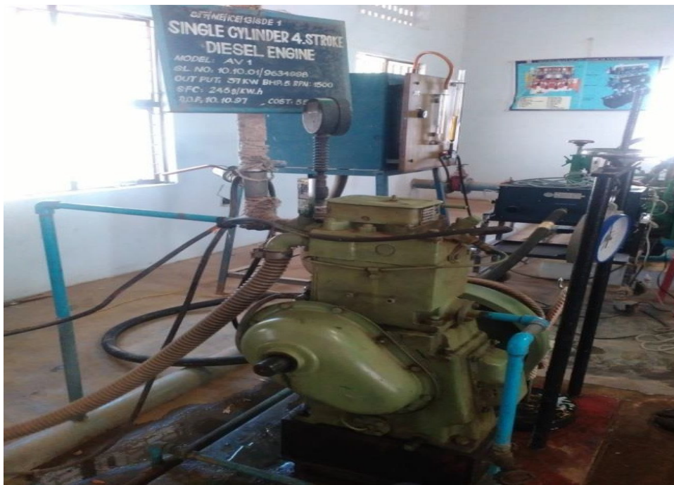
Figure – 3 Single cylinder 4 stroke diesel engine.
