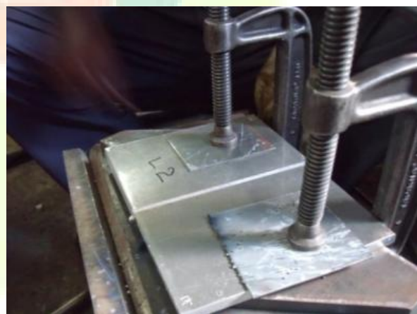
Fig.5. Clamping arrangement
