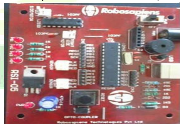
Fig 5.Atmega 8 Controller board
