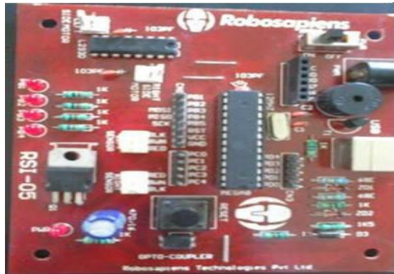
Fig 5. Atmega 8 Controller board
