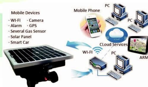
Fig. 1: In this figure, smart monitoring car on the left is shown as one type of mobile sensing nodes, which is developed by our lab. This smart car is equipped with various sensors, e.g., CO, SO<sub>2</sub>, H<sub>2</sub>S, humidity, video and audio sensors. It is connected with control platform and remote server for comprehensive on-line monitoring in petrochemical plants.
