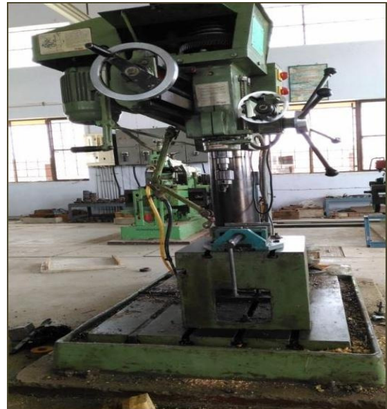
Figure1: Radial Drilling Machine
