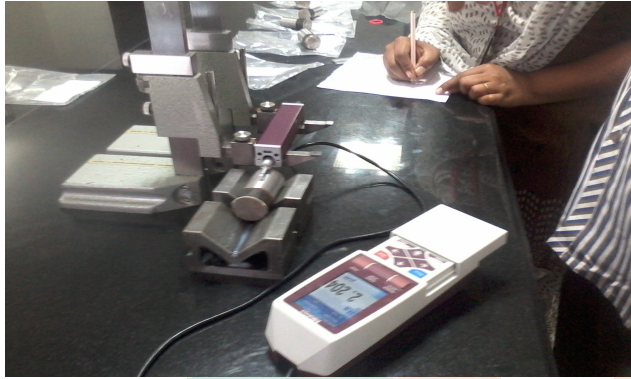
Figure 3: Surface roughness tester used in the experiments
