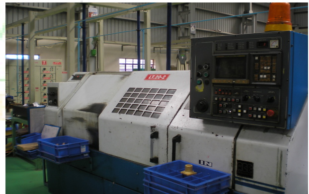
Figure 2: CNC turning machine used for the experiments
