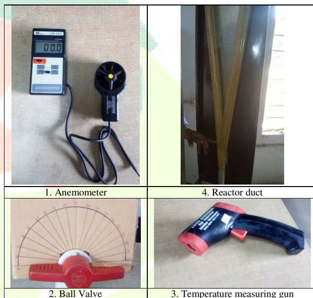
Fig 2.1: Apparatus required for Free-fall Experiment
