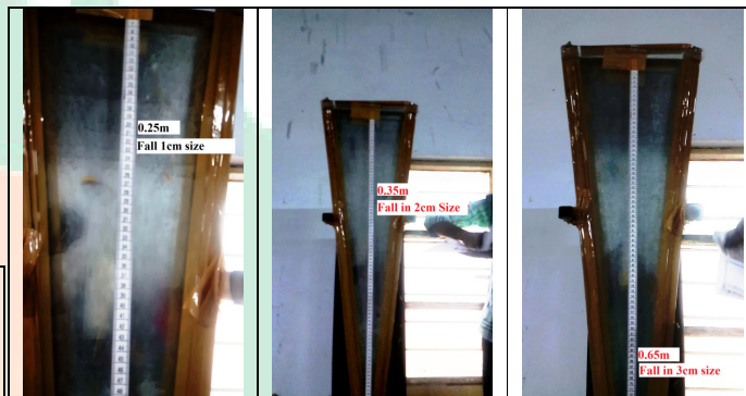
Fig 3.1: Result of different free falling height
