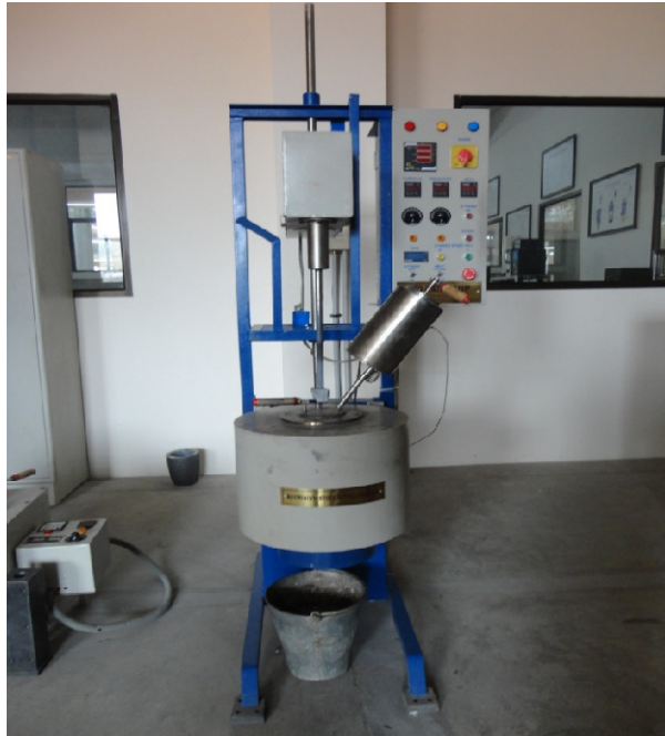
Stir casting setup
