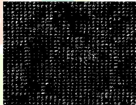
Each eight by eight block is hit with the DCT.
