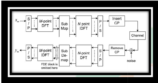
In OFDM frameworks, as the pilot just possess some piece of aggregate subcarriers, we can just get the evaluation of halfway recurrence reaction, which is indicated as
