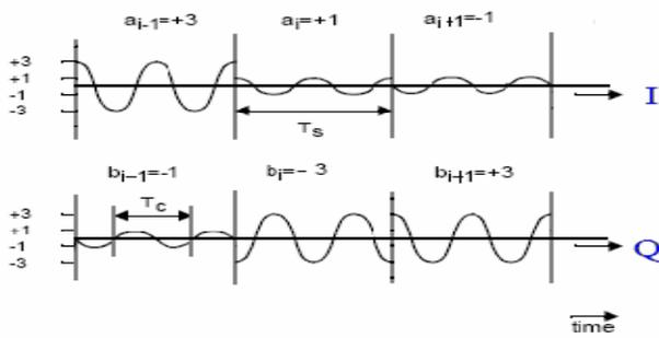
and two bits for Q. The 16 symbols in the constellation diagram are equally spaced and independent, and each is represented by a unique combination of amplitude and phase.
