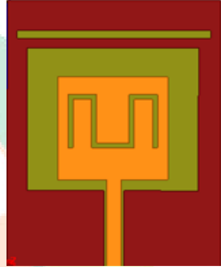
Figure 1 Geometry of wearable patch antenna with two U-shaped connected slots
