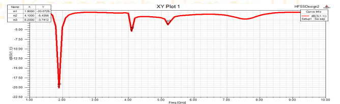
Figure 2 Return loss curve of wearable patch antenna with two U-shaped connected slots
