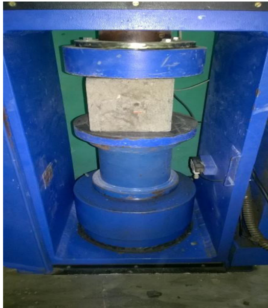
Figure3. Compressive Strength Test
