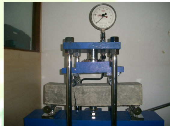
Figure 4. Flexural Strength Test
