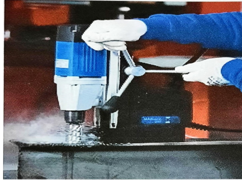
Fig 4 shows the magnetic drill machine
