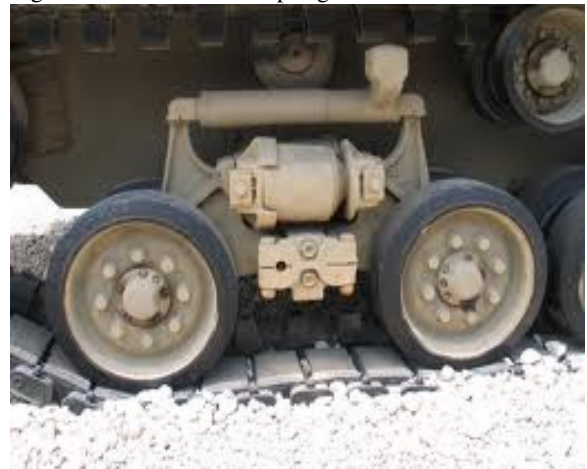
Figure 2. Photo of horizontal springs
