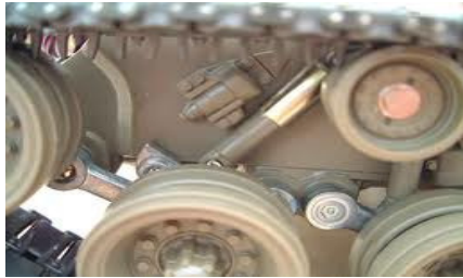
Figure 3. Photo of existing torsion bar
