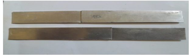
Figure 5 – Joint configuration
