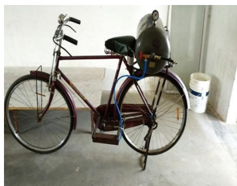
Fig 4.1 Air Pressure Cycle
