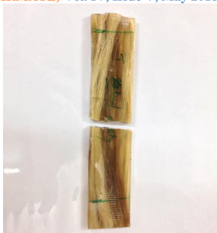
Fig 6 Tensile test specimen Fig 7 Tensile values of specimen
