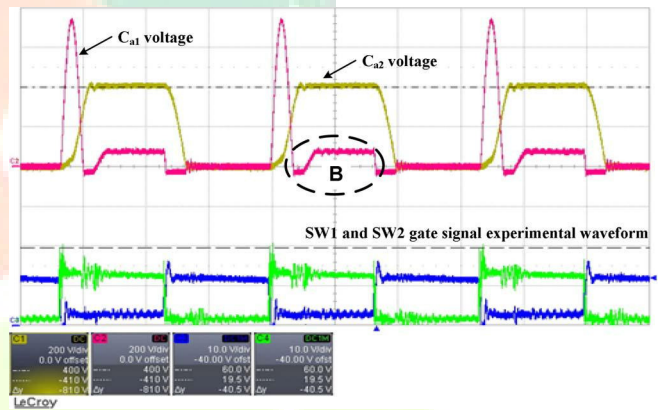
Fig. 13. Experimental results of voltage waveforms of C_{a1} , C_{r1} , and switching signals ( C_{a1} and C_{a2} voltage; Y-axis: 200 V/division, gate signal; Y-axis: 10 V/division, X-axis: 10 \mu s/division).
