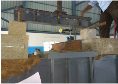
Figure 4.14 Deformation of Top tubular Delta Hollow Flange beam with web stiffener
