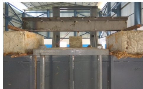
Figure 4.13 Deformation of Top tubular Delta Hollow Flange beam without web stiffener
