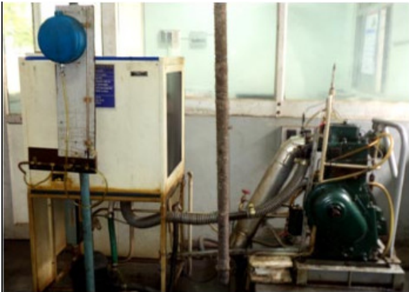
Figure-2 Engine setup for performance and emission tests.
