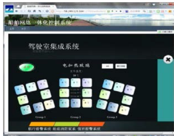
Fig. 5 Ship Equipment Monitoring and Control System Testing Platform
