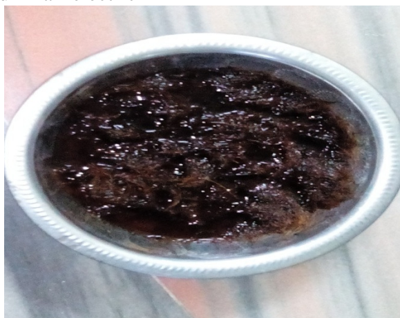
Figure 1 NaOH treatment of coir fiber
