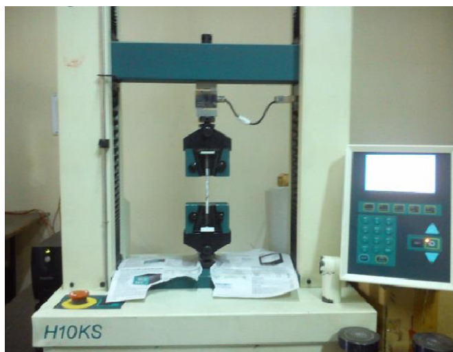
Figure 7 Tensile Test
