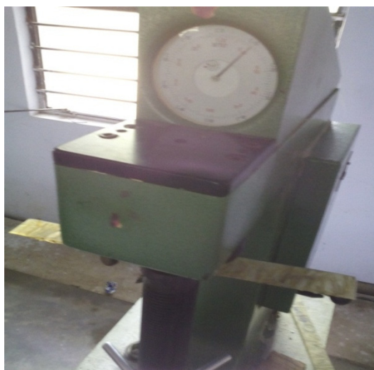
Figure 8 Rockwell hardness setup
