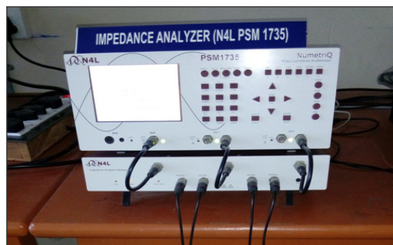
Figure-3 Photo graph of the setup of the commercial impedance analyzer
