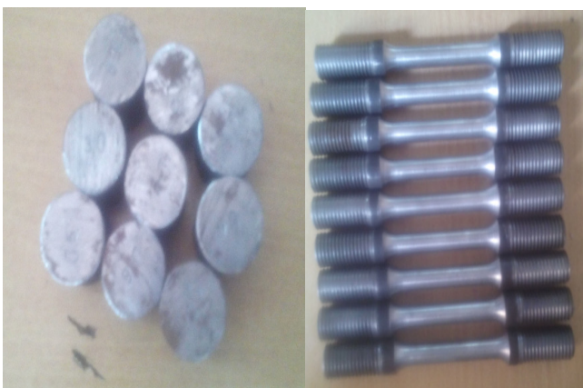
Fig 2 Specimens prepared for Hardness and Tensile test
