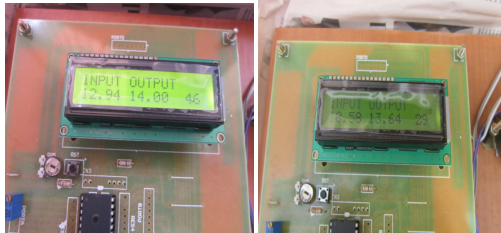
Fig.16 Output of the Cuk converter obtained in both buck and boost mode
