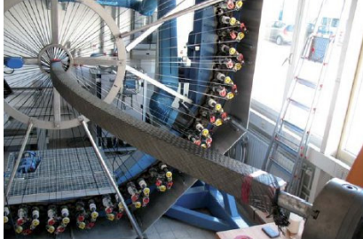
Figure 8: Construction of CFRP sandwich beam [78]
