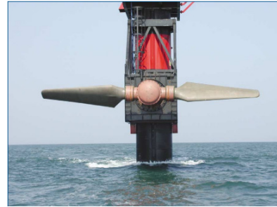
Figure 3: The 300kW Seaflow system installed off Lynmouth [31]
