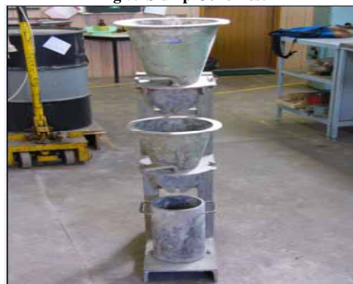
Fig 5.2 Compacting Factor Test
