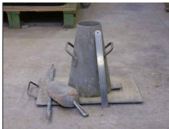
Fig 5.1 Slump Cone Test
