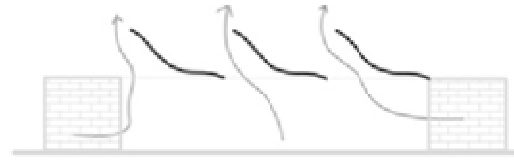
Figure 5. Ventilation provided by module rotation
