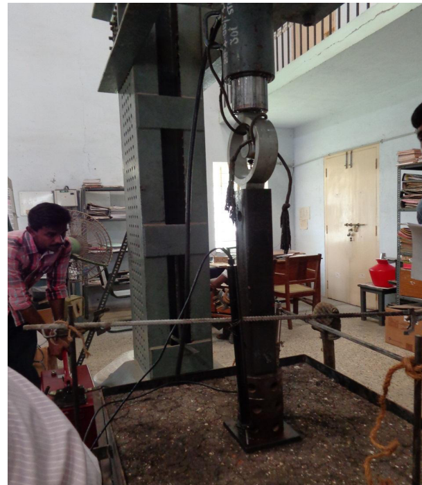
Fig 3 Entire Loading Setup
