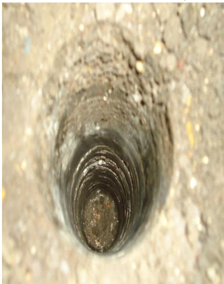
Fig 4 Clay Soil Removed Using GI Pipe
