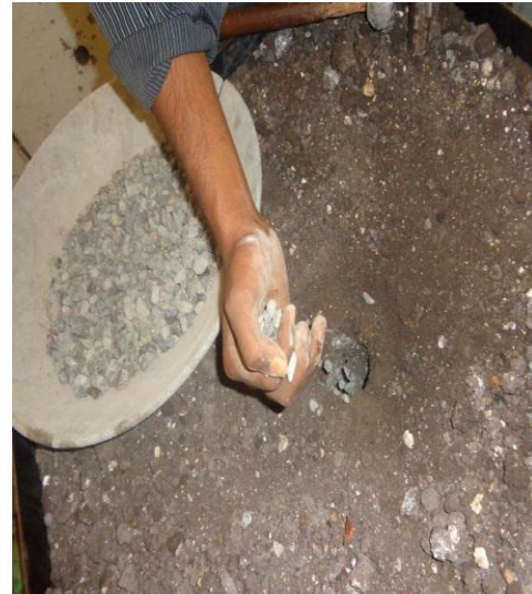
Fig 4a Filling Coarse Aggregate
