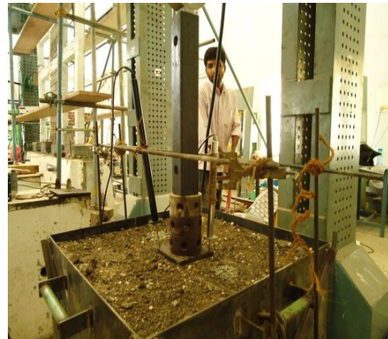
Fig 4B Three Full Stone Columns Testing
